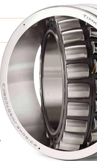
**Optimized Efficiency** - Eliminating the center guide ring also reduces running torque up to 4%. Without a guide ring, less friction is created, meaning less energy is needed to move the bearing and keep it moving. This leads to improved efficiency.
